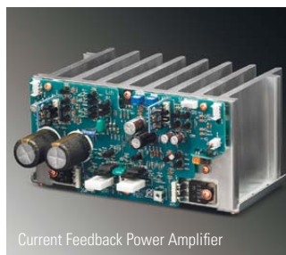
Customized Block Capacitors with 20,000µF each
