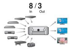
For connection to a broad range of digital sources, this unit features 8 HDMI inputs, including 1 on the front panel that lets you quickly and conveniently connect a camcorder, game console or other HDMI-equipped device. There are dual HDMI outputs for the main room, and a third HDMI output for another room.
