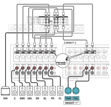
\* The top front or top rear speakers can be connected instead of the top middle speakers. In this case, set the ceiling speakers to be connected under "Height" - "Layout" in the menu. ( p. 243)
