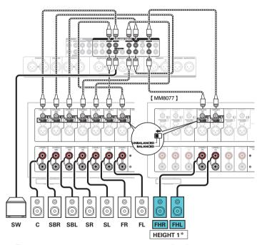
\* The rear height speakers can be connected instead of the front height speakers. In this case, set the height speakers to be connected under "Height" - "Layout" in the menu. (12) p. 243)
