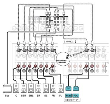
\* The surround Dolby speakers can be connected instead of the front Dolby speakers. In this case, set the Dolby Atmos Enabled speakers to be connected under "Height" - "Layout" in the menu. ( 19 p. 243)
