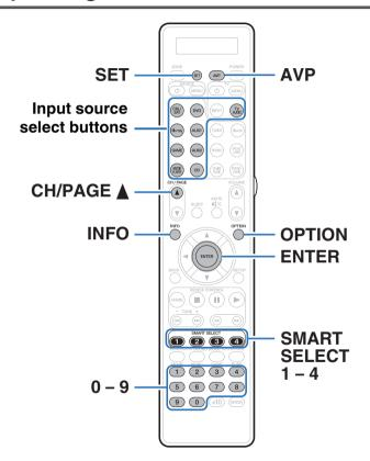
When preset codes are registered in the included remote control unit, it can then be used to operate any devices you have, such as DVD players or TVs made by different manufacturers.
