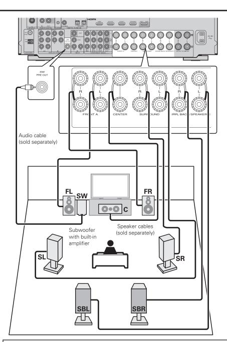
The "Simple version" section provides the speaker installation, connection, and setup methods for the 7.1-channel system with surround back speakers. For the installing, connecting, and setup methods of speakers other than the 7.1-channel system (with surround back speakers), see page 30.
