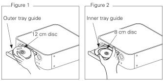
• Place 8 cm discs in the inner tray guide without using an adapter.
