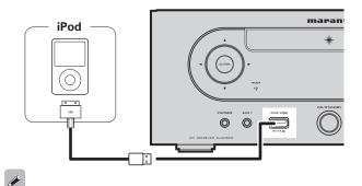
To connect an iPod to this unit, use the iPod cable supplied with the iPod.
