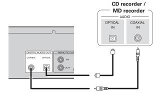
When connecting the optical digital output connector with an optical transmission cable (sold separately)
