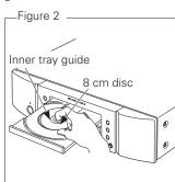
• Place 8 cm discs in the inner tray guide without using an adapter.
