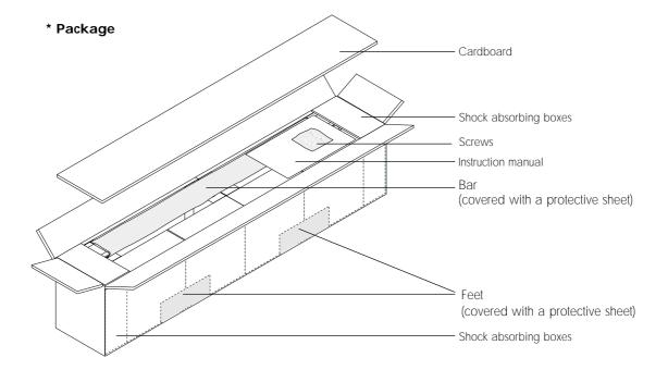
2. Take out the bar and remove the shock absorbing boxes from both sides.
