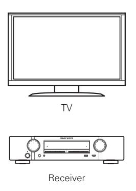
☐ Connect the receiver to your TV with an HDMI cable.
