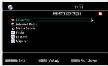
• When in device control mode, REMOTE CONTROL is displayed on the television screen of the controlling device, and REMOTE is displayed on the television screen of the device being controlled.
