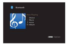
When using for the first time, the unit will go into the pairing mode automatically and "Pairing..." will appear on the display of the unit.
