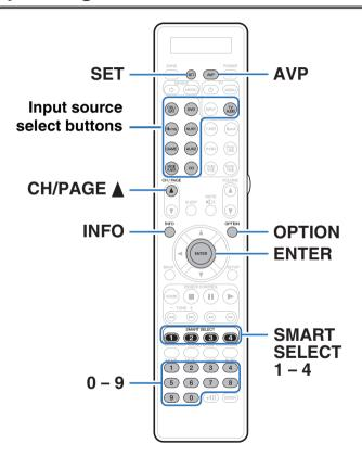
When preset codes are registered in the included remote control unit, it can then be used to operate any devices you have, such as DVD players or TVs made by different manufacturers.
