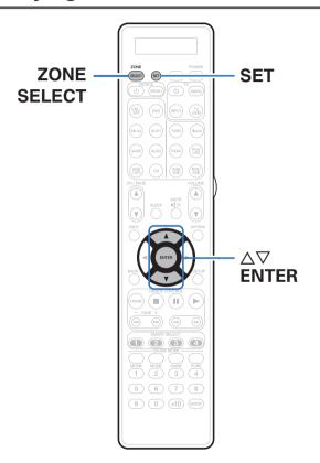
When the ZONE SELECT is pressed, only the set zone can be operated with the remote control unit.
