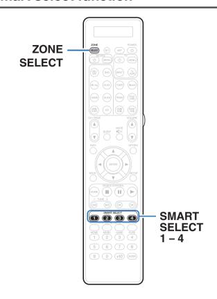
Settings such as the input source, volume level and sound mode can be registered to the SMART SELECT 1 - 4 buttons.
