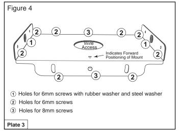
Attach Horizontal Tilting Plate 3 to the previously combined plates (already installed on ceiling) using the two (2) 8 (mm) screws and four (4) 6 (mm) screws provided, as indicated in Figure 4. Install two (2) 6 (mm) screws with rubber spacers and metal washers into the welded metal studs (indicated #1).
