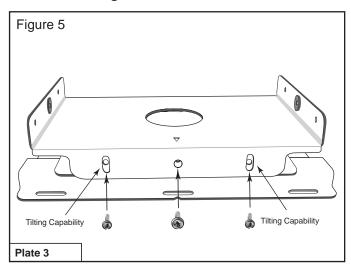
The newly combined Plate 3 provides 10<sup>0</sup> degrees of horizontal tilt. When positioned, tighten with screws provided.
