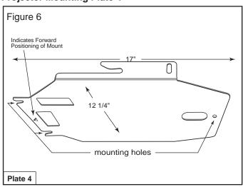
Invert the projector and place it on a soft and flat surface. Align the three (3) rubber spacers provided with the three (3) 6(mm) mounting holes on the projector and secure with three (3) 6(mm) screws provided.
