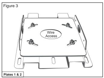
Install the combined plates (above) securely to the ceiling structure in accordance with local commercial building standards.
