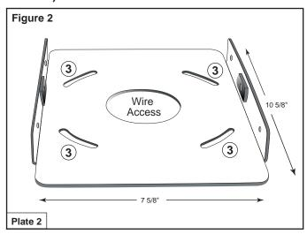
Base plate connector holes #3 provide 15 degrees of horizontal rotation adjustment.
