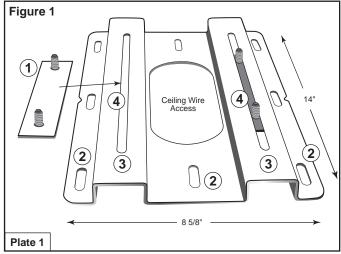
Base Plate Connectors #1 Projector Mount Ceiling Plate 1
