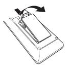
Load the two batteries properly as indicated by the marks in the battery compartment.
