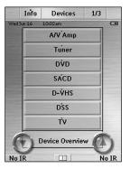
When you jump to a Device by tapping the device button in the Device Overview pages, the RC9500 will change the input of your home theater receiver/preamp.
