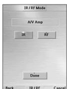
When you have several RX-77s to operate Back IR/RF Cancel devices, you have to assign the correct Extender ID to the selected device. Continue with Step 5.
