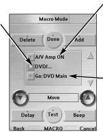
**A/V Amp ON** - When a device name and a button name are listed, that particular button's IR command will be issued.
