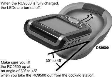
**Note** Normal charging time is 2 to 3 hours, depending on the condition of the battery pack.
