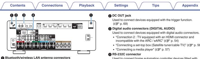
Used to connect the included external antennas for Bluetooth/wireless connectivity when connecting to a network via wireless LAN, or when connecting to a handheld device via Bluetooth. (Pr p. 65)
