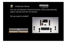
• This feature adjusts the output volume to the optimal level while constantly monitoring the level of the audio input to the unit. Optimal volume control is performed automatically without any loss in the dynamism and clarity of the sound when, for example, the volume suddenly increases for commercials shown during television programs.
