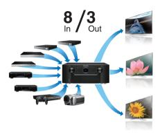
For connection to a broad range of digital sources, this unit features 8 HDMI inputs, including 1 on the front panel that lets you quickly and conveniently connect a camcorder, game console or other HDMI-equipped device. There are dual HDMI outputs for the main room, and a third HDMI output for another room.
