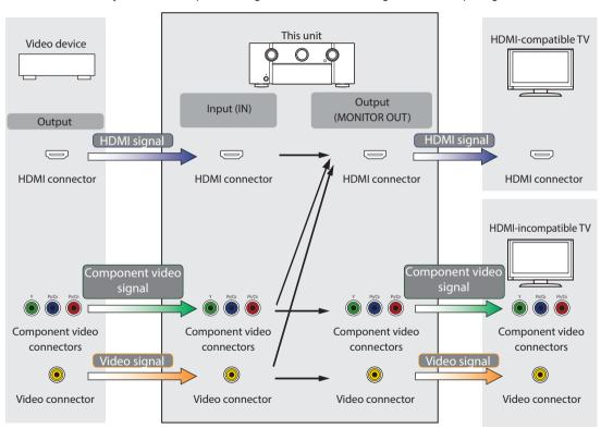
The main zone video conversion function is compatible with the following formats: NTSC, PAL, SECAM, NTSC4.43, PAL-N, PAL-M and PAL-60.
