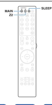
You can have the power automatically switched to standby once a set time has elapsed. This is convenient for viewing and listening while going to sleep. The sleep timer function can be set for each zone.
