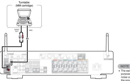
• The earth terminal (SIGNAL GND) of this unit is not for safety grounding purposes. If this terminal is connected when there is a lot of noise, the noise can be reduced. Note that depending on the turntable, connecting the ground line may have the reverse effect of increasing noise. In this case, it is not necessary to connect the ground line.
