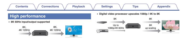
When 8K Ultra HD (High Definition) is used, an input/output speed of 60 frames per second (60p) is achieved for video signals. When connected to 8K Ultra HD and 60p video signal input compatible TV, you can enjoy the sense of realism only available from high-definition images, even when viewing fast-moving video.
