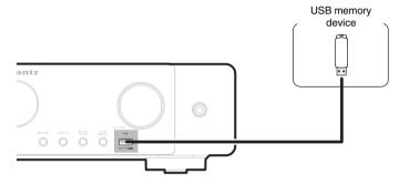
• Marantz does not guarantee that all USB memory devices will operate or receive power. When using a portable USB hard disk drive (HDD) which came with an AC adapter, use that device's supplied AC adapter.
