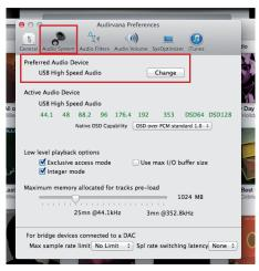
Select USB High Speed Audio, this is the NA-11S1. This will only appear if the NA-11S1 is connected and set to PC input.
