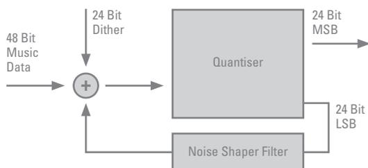
The noise shaper filter only acts with the LSB (the least significant bit, the “smallest” bit) and returns it to the input of the quantizer
