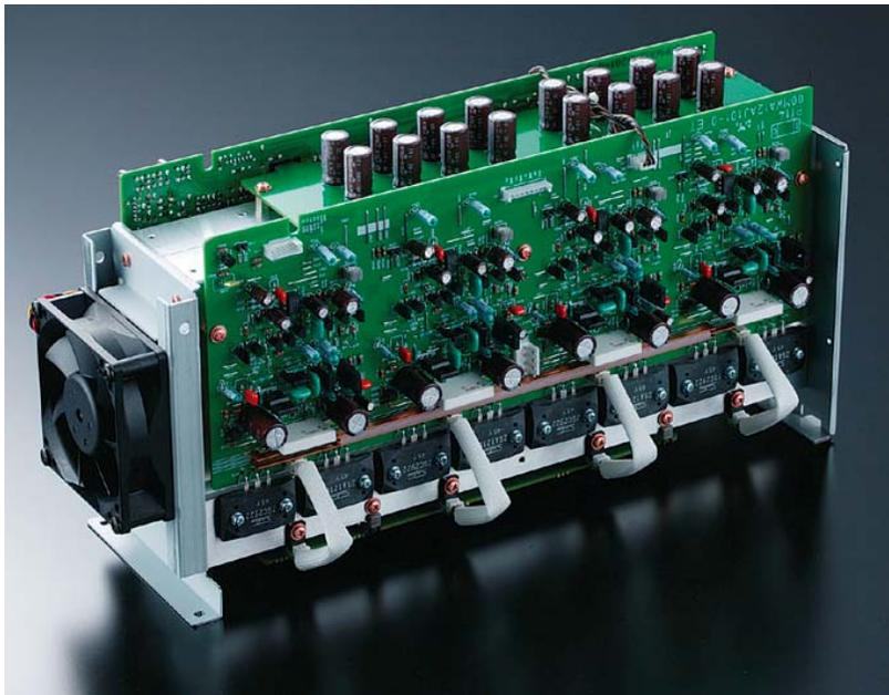
This highly efficient amplifier design utilizes a “tunnel” type heatsink with an extremely quiet variable speed fan that doesn’t even turn on until serious heat occurs. This assures the owner of audiophile level silence. The amplifier uses an OFC copper rail for the power supply side of the output transistors as well as specially sourced OFC cables for the power supply and the speaker outputs.
