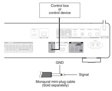
• To use the FLASHER IN jack, set the EXTERNAL/INTERNAL switch to "INTERNAL".
