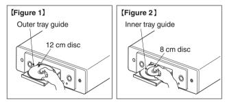
• Place 8 cm discs in the inner tray guide without using an adapter.
