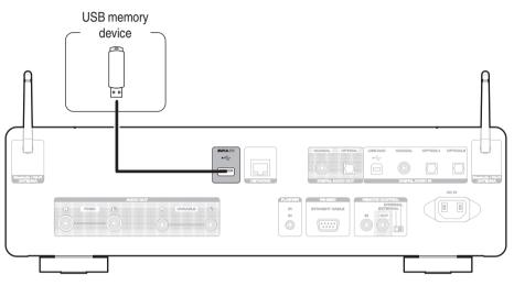
• Marantz does not guarantee that all USB memory devices will operate or receive power. When using a portable USB hard disk drive (HDD) which came with an AC adapter, use that device's supplied AC adapter.
