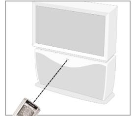
You can choose to operate devices using radio frequency (RF) signals instead of IR signals. RF signals have an operating distance of approximately 20 meters (66 feet) in house and can, unlike IR signals, go through obstacles like furniture or walls.
