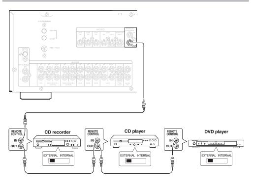
You can control other Marantz products through this unit with the remote control by connecting the REMOTE CONTROL terminals on each unit.
