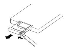
② Load the battery case with the provided battery, insert the battery correctly according to the "+" indication on the battery case then slide the battery case into the remote control unit it clicks.
