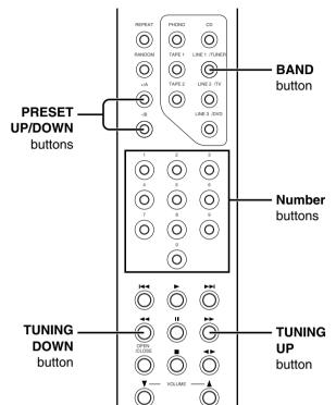
Press the LINE 1/TUNER button to switch the input selector of the PM-17.
