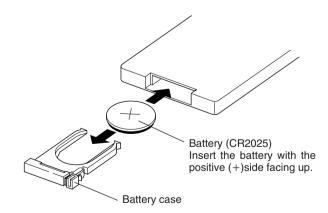
The battery life is about 1 year under normal use. The life is depended on the operating condition. Take the battery out of the unit when it is not to be used for a long period of time.
