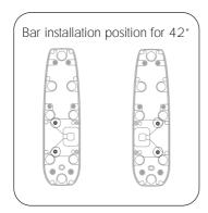
\* For 42-inch plasma displays, the 2 cores, 4 core mounting screws and 2 display mounting screws are not used.
