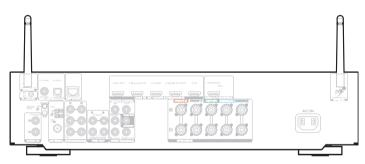
3) Connect the receiver to your TV with an HDMI cable
